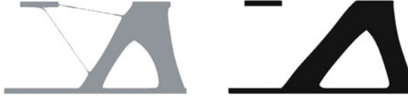
FIGURE 14. In the optimization of the excess probability for \eta = 0.4 decreasingly thin trusses are realized on the intermediate grey shape on the left until the left bearing is completely truncated via a topology optimization step (cf. Fig. 9 for the load configuration). The final result is shown on the right. (Figure reprinted from [25, Fig. 7])
