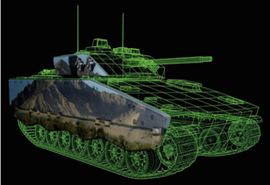
Fig. 3.6 The adaptive E-ink camouflage developed by BEA Systems updates the image portrayed on each side of a tank, making it blend into the background (Image courtesy of BEA)
