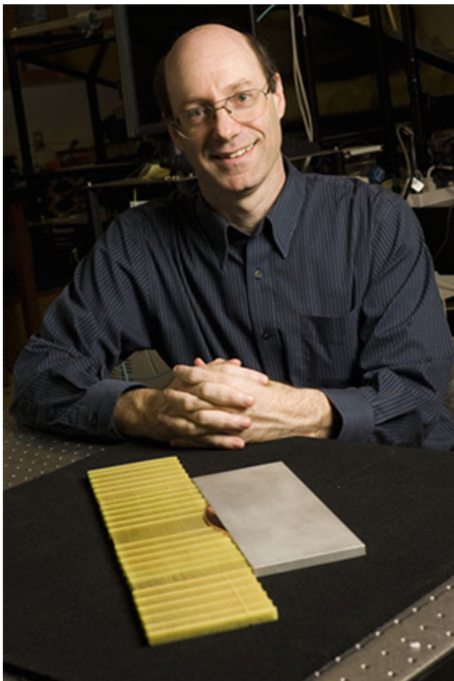
Fig. 5.29 The microwave metamaterial carpet cloak built by researchers at Duke University in 2008. The cloaked region is under the central copper bump – David Smith is pictured in the background (Picture courtesy of Duke University)
