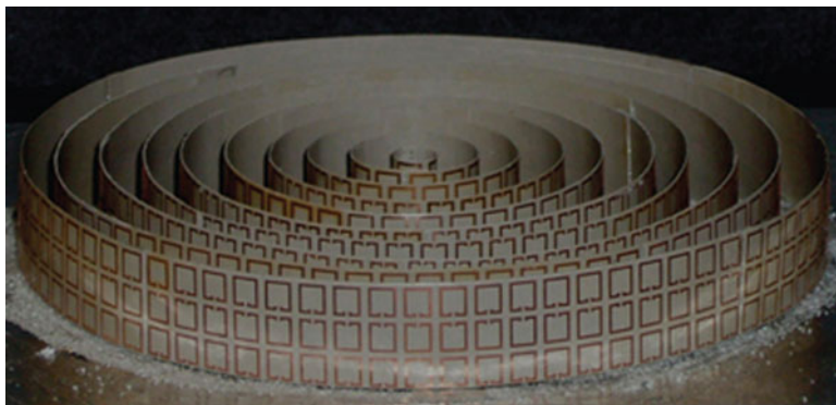
Fig. 3.30 A two-dimensional Eaton lens for microwave radiation. The device is composed of a metamaterial made of copper split-ring resonators etched onto circular mica circuit board substrates. The entire device is 80 mm in diameter (Image from arXiv:0906.5214v1)
