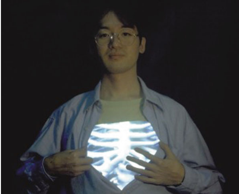
Fig. 3.14 The X'tal (crystal) vision and RPT. In this case an optical image of an X-ray chart is directed towards a retroreflecting shirt, thus enabling the observer to see both a real and a virtual image at the same time
