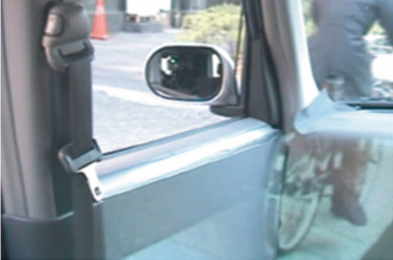
Fig. 3.11 By being able to see through the car door a driver can more accurately gauge the distance to a cyclist or pedestrian (Image courtesy of the Tachi Labs, the University of Tokyo)
