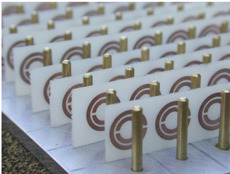
Fig. 5.8 The first purpose-built metamaterial to test the ideas of negative refractive index media as theoretically described by Pendry et al., and Vesalago. Copper loops (split ring resonators) have been etched on to fiberglass circuit board substrates, and the wire and resonator substrates have been arranged into a lattice structure (Image courtesy of University of California at San Diego)
