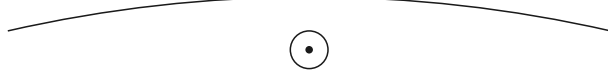
Fig. 3.1. An atom in the field of a light wave with wavelength much longer than the typical extension of the atom
