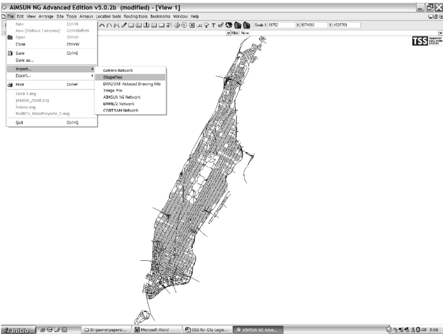
Figure 8-5. Dialogue to import a shape file into AIMSUN NG and the imported digital map (Manhattan).
