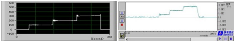
Fig. 3. Comparison of optical fiber dynamic test and electrical method strain time curve
