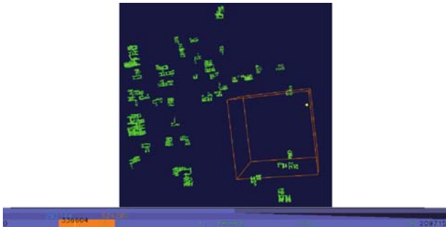
Fig. 5. Effective use of screen real estate. Three annotations of sizes 63, 54, and 63 separated by 565 and 11,260 basepairs, respectively, on 2,097,151-basepair-long sequence are distinctly visible in 3D space ( in orange cube ). But the first two merge in a 1D representation ( in orange rectangle )
