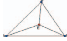
Fig. 6. A grid block divided into three triangles for a piecewise linear approximation of the solution
