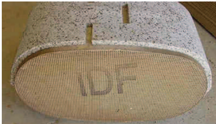
Fig. 2. A ceramic honeycomb catalyst structure of a catalytic converter
