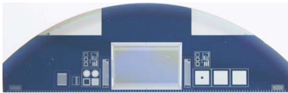
Fig. 1.31 Half-moon with test structures. Left to right , the structures with the following accessible process parameter are located (1) TS-CAP ( C_{coupling} , V_{break} ), (2) sheet (Resistivity Al , Resistivity p+ , R_{poly} ), (3) Gate Controlled Diode (GCD) ( I_{surface} ), (4) CAP-TS-AC ( C_{inter-strip} ), (5) full minisensor, (6) CAP-TS-DC ( R_{inter-strip} ), (7) Diode ( V_{FD} ), (8) MOS1 ( V_{flat-band} ), (9) MOS2 ( V_{flat-band} )
