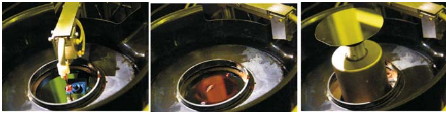
Fig. 1.37 Photoresist is roughly spilled in the middle of the wafer, centrifugal forces, during fast rotation, homogeneously distributes the resist on the wafer. Courtesy of ITE Warsaw [156]
