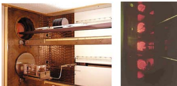
Fig. 1.35 Two quartz tubes in the furnace are visible on the left photo including the loader of several wafers. Each individual furnace has a well-defined atmosphere and always remains at the same temperature and content mixture. There is one furnace for each individual process. On the right , several burning furnaces are shown. Courtesy of ITE Warsaw [156]
