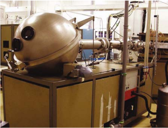
Fig. 1.40 The picture shows an ion implanter. Ions are accelerated and guided onto the target inside the sphere, where several wafers are rotated and homogeneously hit. The ions do not penetrate through the masking layer ( \text{SiO}_2 or photoresist), therefore well-defined patterns, e.g. strips/pixel can be implemented on the wafer. Courtesy of ITE Warsaw [119, 156]
