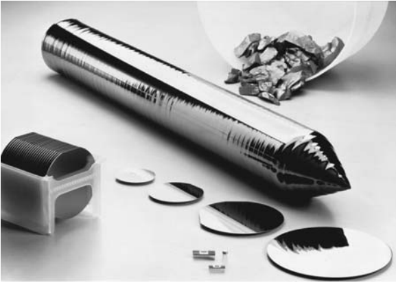
Fig. 1.33 A silicon ingot, source of about 200 wafers. The picture shows raw silicon chips, a full size silicon ingot and sliced silicon wafers of different size. [Copyright Sitronic AG]
