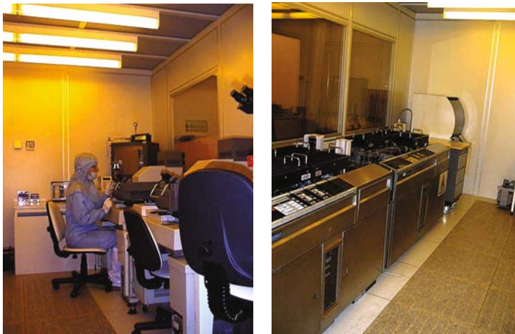
Fig. 1.38 On the left the mask-aligner is printing the mask onto the photoresist with UV light, opening the windows for the next etch process step. On the right, the spinner and developing machine can be seen. Courtesy of ITE Warsaw [156]
