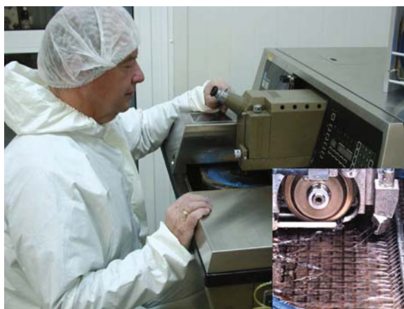
Fig. 1.47 The cutting of chips with a diamond saw. Note the high water flux to avoid heating up due to the high rotation speed. Courtesy of ITE Warsaw [156]
