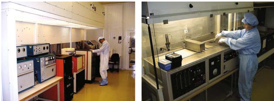
Fig. 1.39 On the left , the plasma etching laboratory of a silicon plant in an institute is shown. On the right , the wet etching facility is displayed. The secret and art lies in the special recipes to use the right acid, the right duration and time on the different structures and materials, like Si, \text{SiO}_2 and Al. Courtesy of ITE Warsaw [156]
