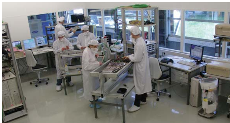
Fig. 5.26 Petal integration in Karlsruhe. Three technicians plus two physicists were assembling two petals simultaneously. The petals were mounted on so-called petal grills which enable easy turnaround and thus access to both sides. After assembly, petals were long-term tested in fridges with additional active petal cooling
