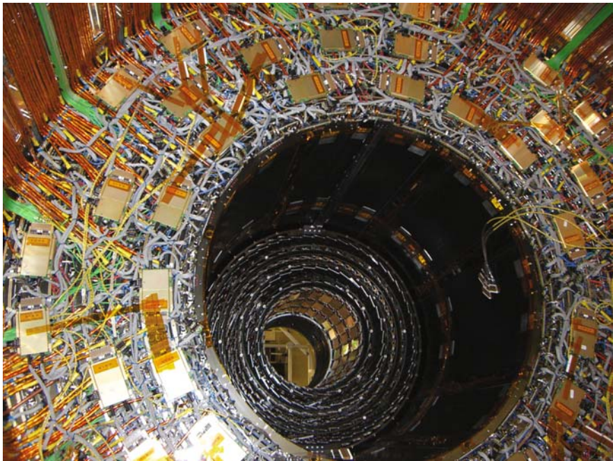
Fig. 5.9 TIB inserted in TOB, a rare view. The four layers of the tracker inner barrel are visible inside the tracker outer barrel. The TOB layers 5–10 are completely hidden by the necessary cabling. This is a rare view during the time of construction
