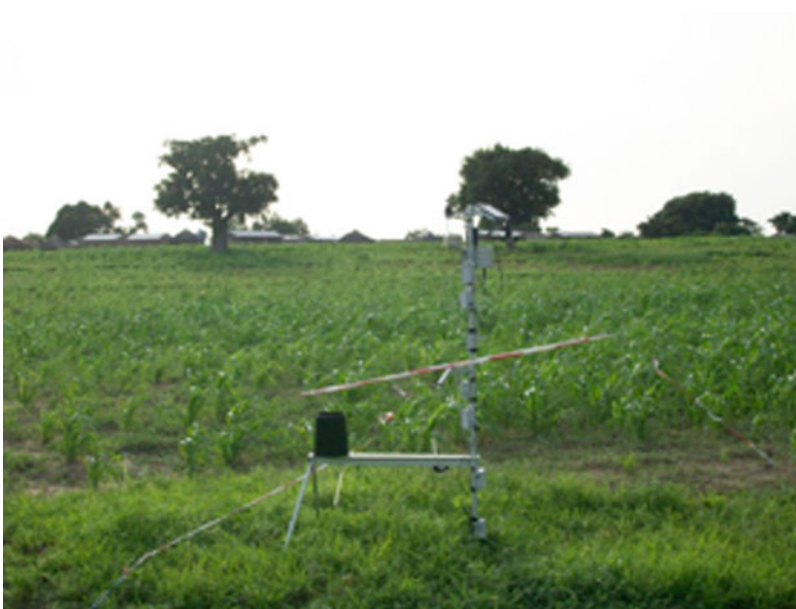
Fig. 15.1 Wireless sensing device, Sensorscope' used for observation in agricultural field
