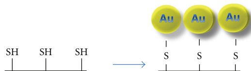
FIGURE 1: Chemical attachment between S–H and gold (Au): on the left the original thiol molecule and on the right the gold particles chemically bounded to the thiol molecules.
