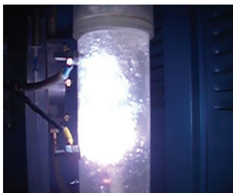
FIGURE 4: Typical photograph of multispark discharger operating in water.
