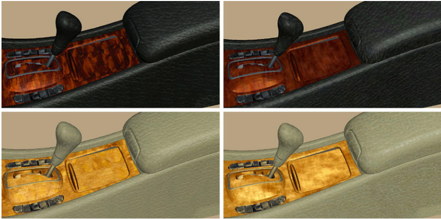
Fig. 14.5 BTF measurements mapped on part of a car gearbox. Original BTF data (enlarged using image tiling) ( left ) compared with synthesized BTF ( right ) for four distinct materials: wood01 , foil01 , wood02 , foil02 (3D model courtesy of DaimlerChrysler)
