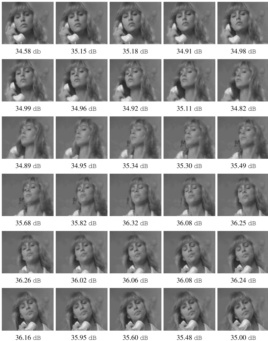
Fig. 6.7 Suzie. Reconstruction of video data by our approximation method 3AT . The reconstruction is represented by 30 consecutive image frames, displayed from top left to down right . For each image frame, the corresponding PSNR value is shown
