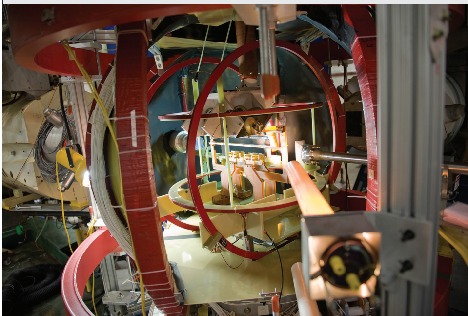
FIGURE 2.5.1 Photograph of JLAB's polarized helium-3 target, used to make precision electron scattering measurements of the charge, magnetism, and spin distributions of the neutron. SOURCE: Courtesy of JLAB.
