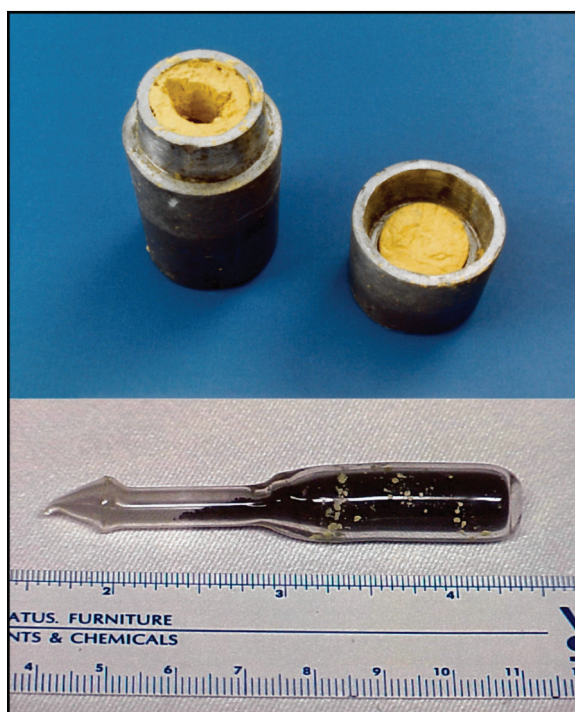
FIGURE FOR 1 Lead container and the glass ampoule containing highly enriched ^{235}\text{U} seized in Bulgaria in 1999 and analyzed at Lawrence Livermore National Laboratory for forensic purposes. SOURCE: “Forensic Analysis of a Smuggled HEU Sample Interdicted in Bulgaria,” UCRL-ID-145216, August 2001.
