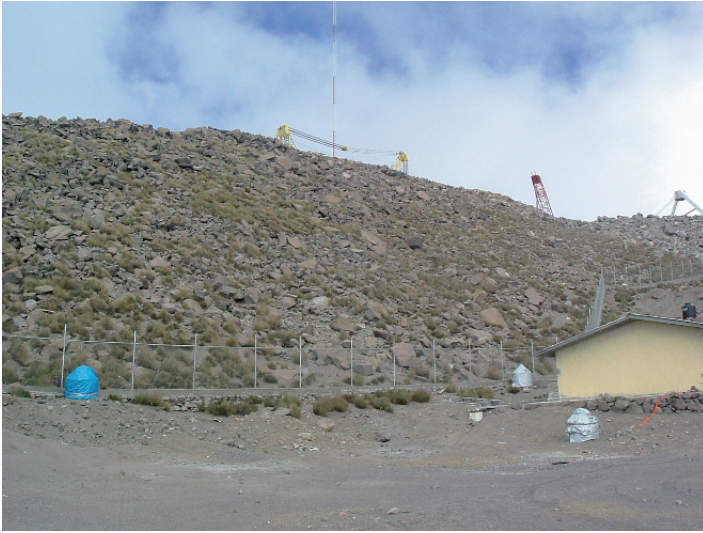
Fig. 1. Sierra Negra Array site, showing 3 light-tight cylindrical water Cherenkov tanks.
