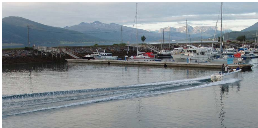
Fig. 6 Waves from a small boat entering Nesna harbour (Norway, north of Mosjoen) at a supercritical speed.
