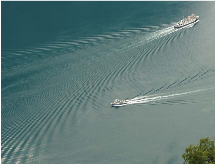
Fig. 2 Pattern of ship waves in Geirangerfjord, Norway.
