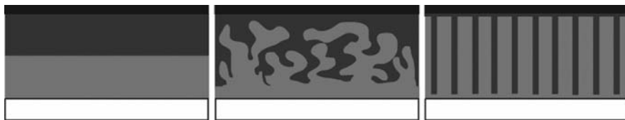
Fig. 11.3 Architectures of typical organic solar cells. Planar bilayer heterojunction ( left ), disordered bulk heterojunction ( center ) and ordered bulk heterojunction ( right )
