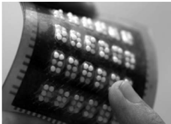
Fig. 7.18 An image of the Braille sheet display which is manufactured on a plastic film integrating the active matrix of organic transistors with polymer actuator array based on a perfluorinated polymer electrolyte membrane. The device is a thin, lightweight, and flexible sheet Braille display. From Fig. 7.1 in Ref. [23] ((c) 2008 IEEE)
