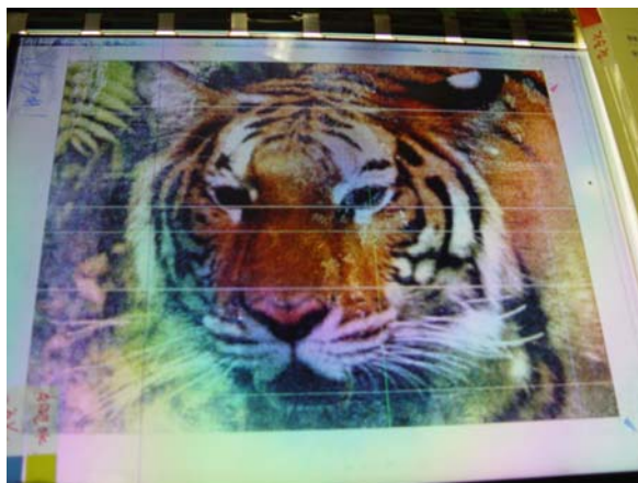
Fig. 8.10 A 15" diagonal XGA (1024×768) color LCD using pentacene TFTs on glass. From Ref. [31]. Permission for Reprint courtesy Society for Information Display
