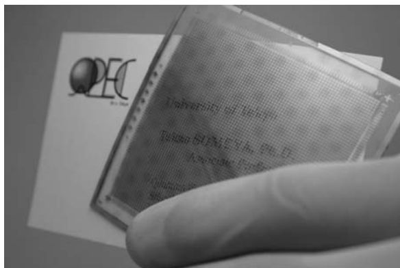
Fig. 7.1 An image of a large-area, flexible, and lightweight sheet-type image scanner placed onto the business card for capturing images. The effective scanning size is 50 \times 50 \text{ cm}^2 and the resolution is 36 dpi. From Fig. 7.1 in Ref. [18] ((c) 2008 IEEE)
