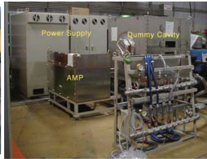
Fig. 23. RF core made of metal alloy ( left ). Power supply and amplifier for PRISM-FFAG RF ( right ).
