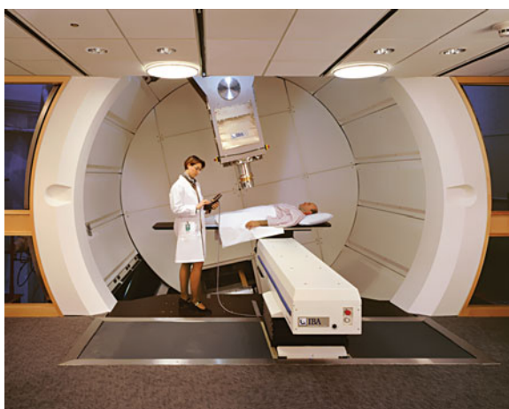
Fig. 35.2 View of a treatment room with gantry, including the beam delivery nozzle ( hanging from above ) and the patient positioning system (PPS)
