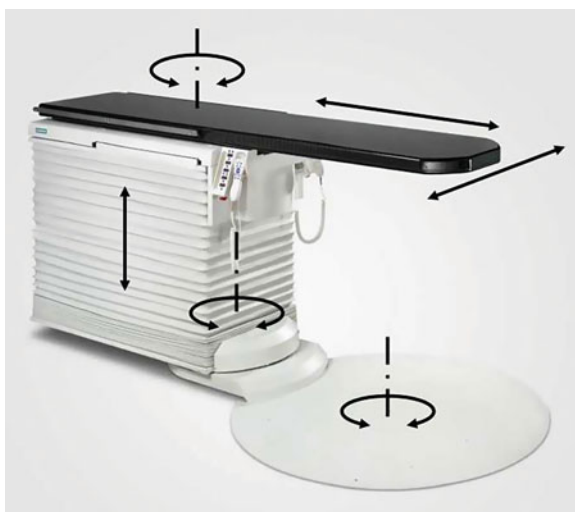
Fig. 33.1 Present-day treatment table for conventional RT with movement characteristics. The column rotation axis is used to move the table out of the isocenter. This axis is used for extended SSD (source-to-surface distance) treatments. Not all commercial tables share this feature though
