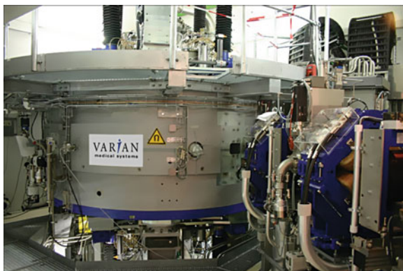
Fig. 23.8 The ACCEL/Varian cyclotron installed at the RPTC in Munich. The beam line with some quadrupoles is visible on the right. Courtesy of Varian Medical Systems
