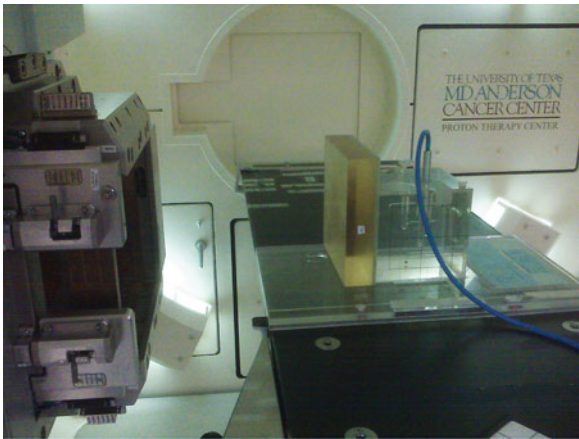
Fig. 28.1 Daily scattered-beam QA point measurements made at proximal, center, distal, and past the spread-out Bragg peak (SOBP)
