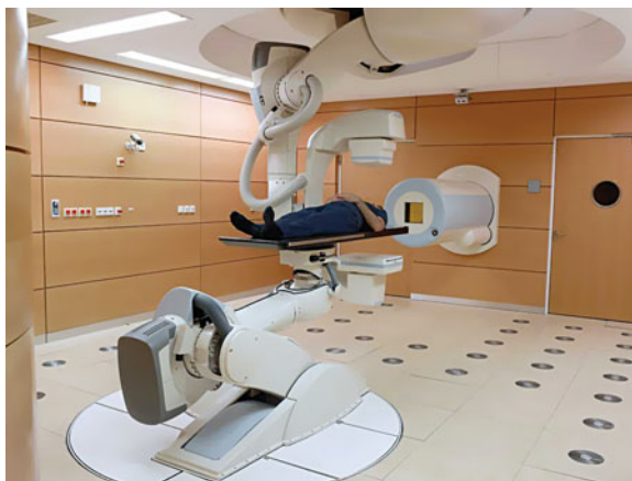
Fig. 33.11 Robots in a treatment room of the HIT facility. The ceiling-mounted robot is used for imaging. In CBCT mode it rotates around the patient. The floor mounted robot positions the patient. The aligned system requires control of 12 degrees of freedom
