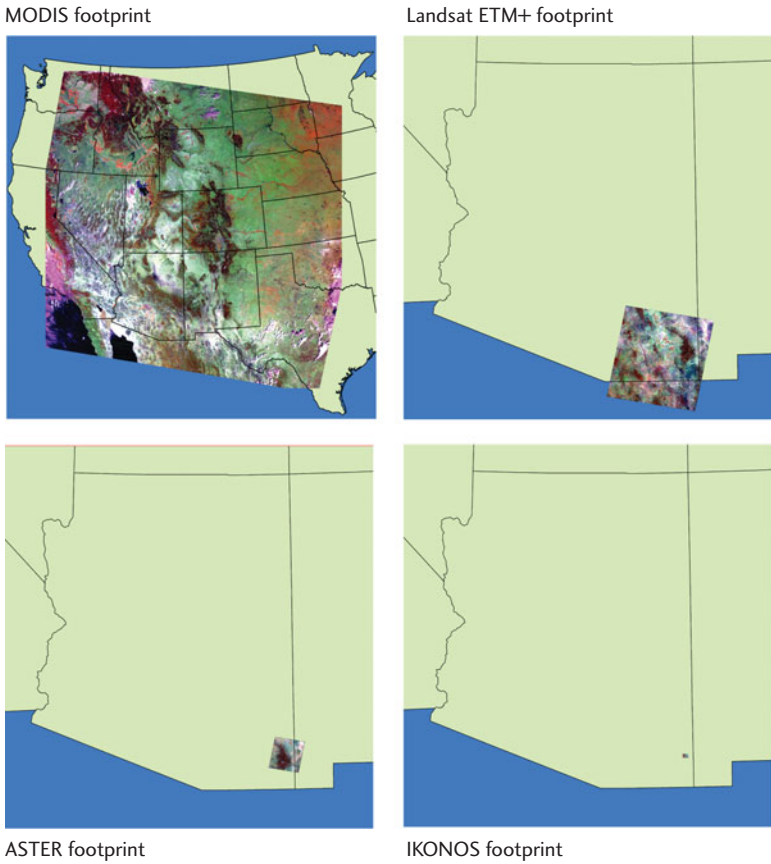
Fig. 2.2 As a general rule, the coarser the resolution of a sensor the larger the footprint will be. The ground widths of the images represented are: MODIS—2330 km, Landsat ETM+—185 km, ASTER—60 km, and IKONOS—11 km. The footprint for the IKONOS image is only a speck at this scale. Credit: American Museum of Natural History’s Center for Biodiversity and Conservation, IKONOS image courtesy of GeoEye.
