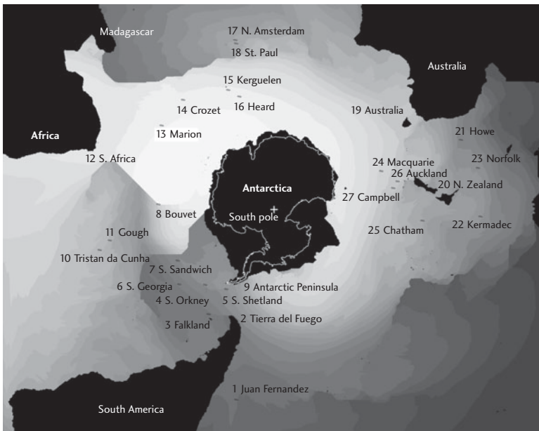
Fig. 8.13 Different gray tones represent different levels of wind connectivity for Bouvet Island (#8), South Atlantic Ocean, as measured by the SeaWinds scatterometer (February 1–10, 2002), with increasing connectivity depicted by going from dark to pale tones. The SeaWinds scatterometer only records wind properties over ocean water surfaces—land surfaces, ocean surfaces covered with ice, and areas with null connectivity values for this time period appear as black due to an absence of data. Figure from Muñoz et al. 2004, with permission from AAAS.
