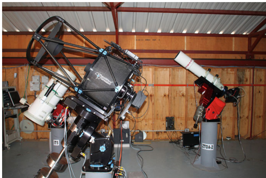
Fig. 6.2 Several iTelescope direct remote control telescopes in roll-off roof observatory (Credit iTelescope)
