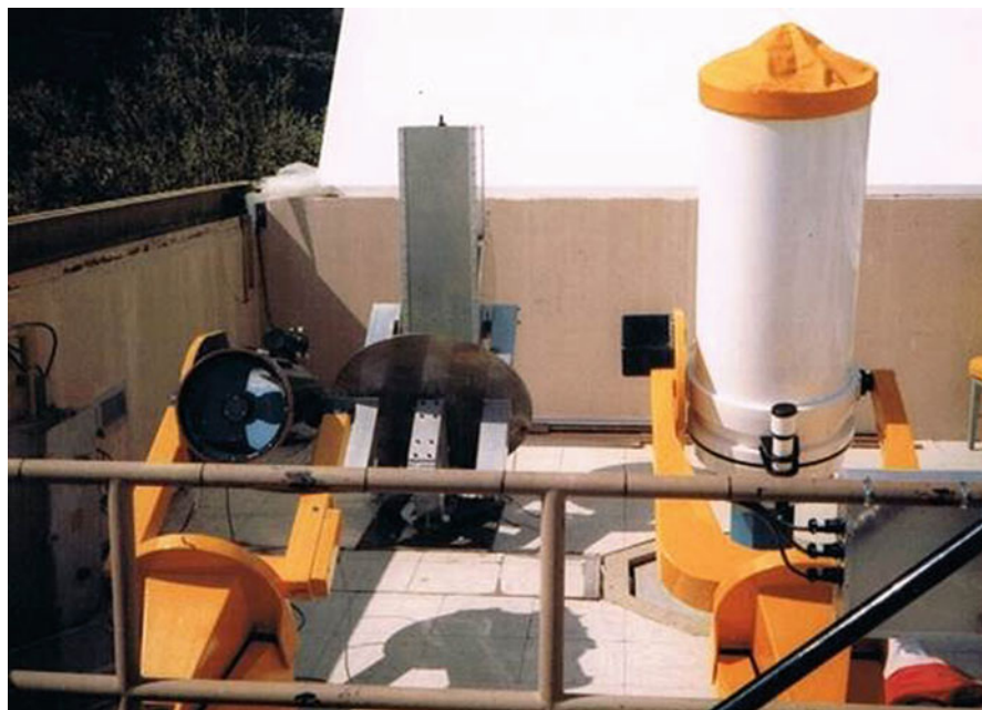
Fig. F4 The original three robotic telescopes at the APT Service on Mt. Hopkins. Left to right: the Fairborn-10, the Phoenix-10, and the Vanderbilt-16
