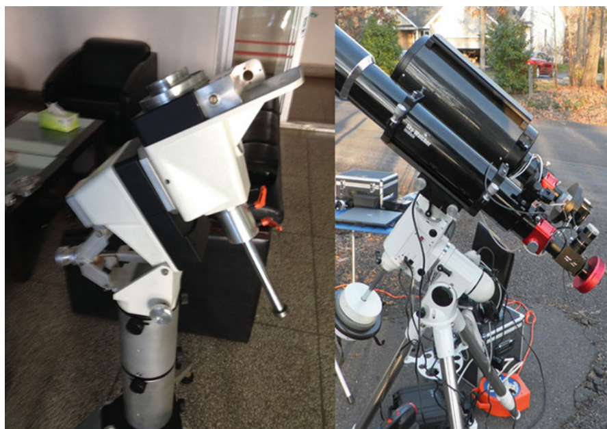
Fig. 3.5 Mount pier and tripod
