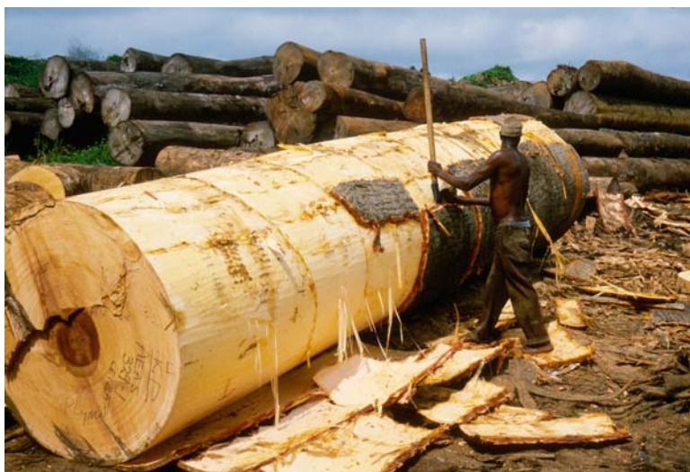
Plate 55 Standard practices in tropical forest harvesting are to peel logs shortly after felling to avoid wood borer attack.
