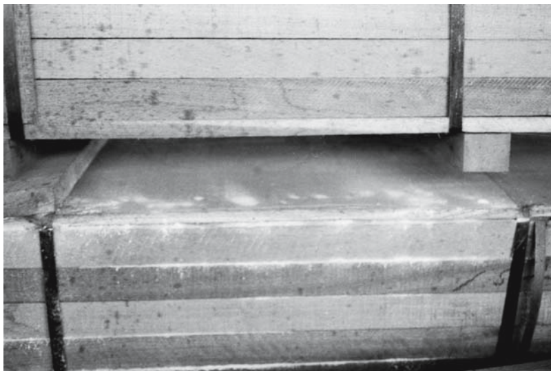
Figure 6.13 Powderpost beetle damage to wawa used in crating high-value odum for export. (Ehwia Wood Products, Kumasi.)
