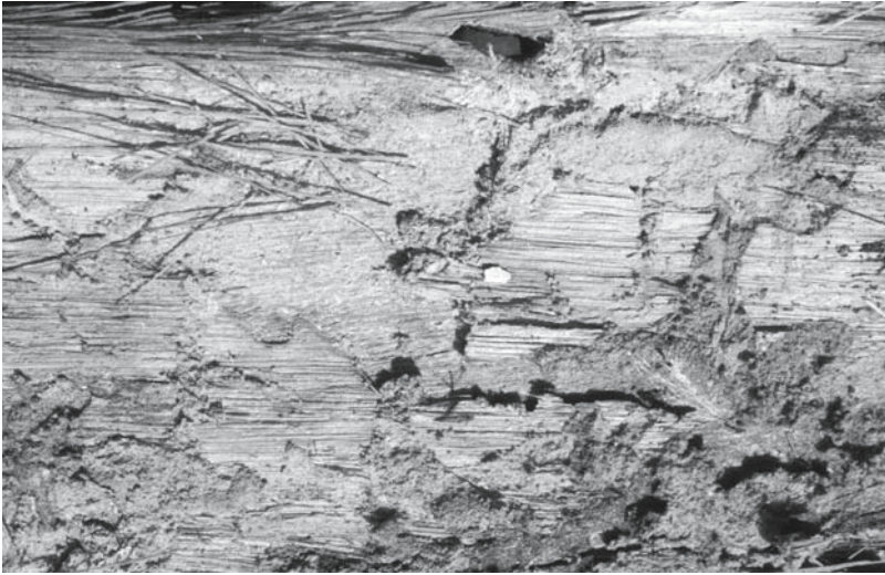
Figure 6.7 Typical evidence of feeding by longhorned wood borers. Note the tightly packed coarse frass in the galleries
