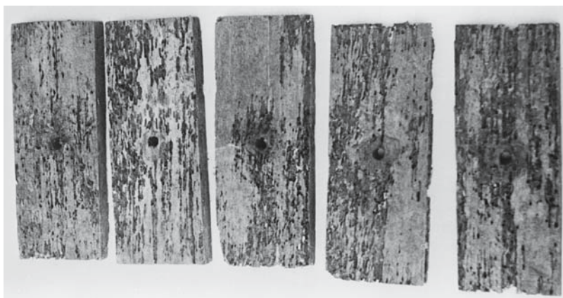
Figure 6.14 Wood damaged by the freshwater wood borer Povilla adusta from Nzulezo in western Ghana. (Photograph courtesy of F.K. Ampong, FPRI, Kumasi.)
