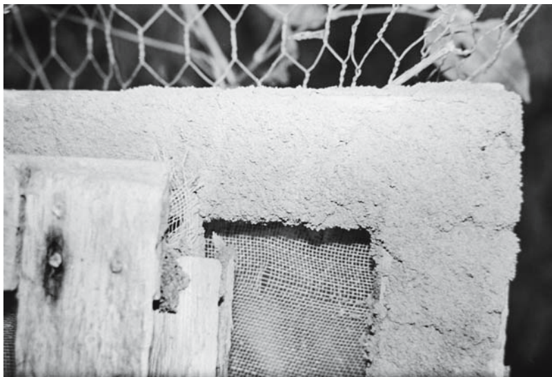
Figure 7.7 Wooden frame left outdoors that is completely covered with earth while the wood is being consumed within
