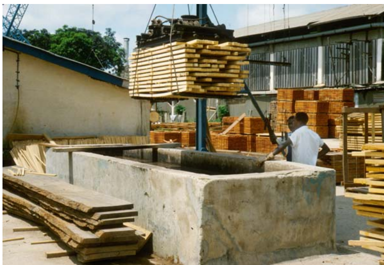
Plate 57 Treating lumber by dipping into tank of wood preservative. Common procedure before export.
