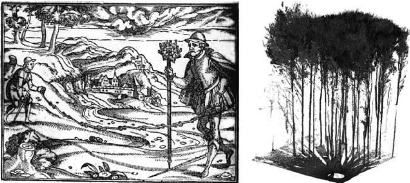
Fig. 1.16 Progressive spatial and temporal refinement of measurements in forests. Forest inventory by means of an ell-chain according to Stephano and Libalto (1598, p. 566) ( left ) and 3D image of the experimental plot Freising 813/2 near Kranzberg by terrestrial laser scanning ( right )
