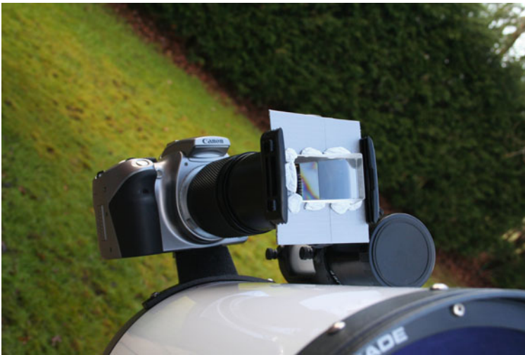
Figure 6.1. Mounting an objective prism.
