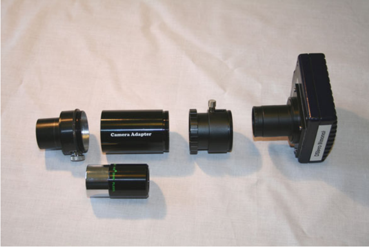
Figure 14.12. Components for adding a transmission grating slit.
