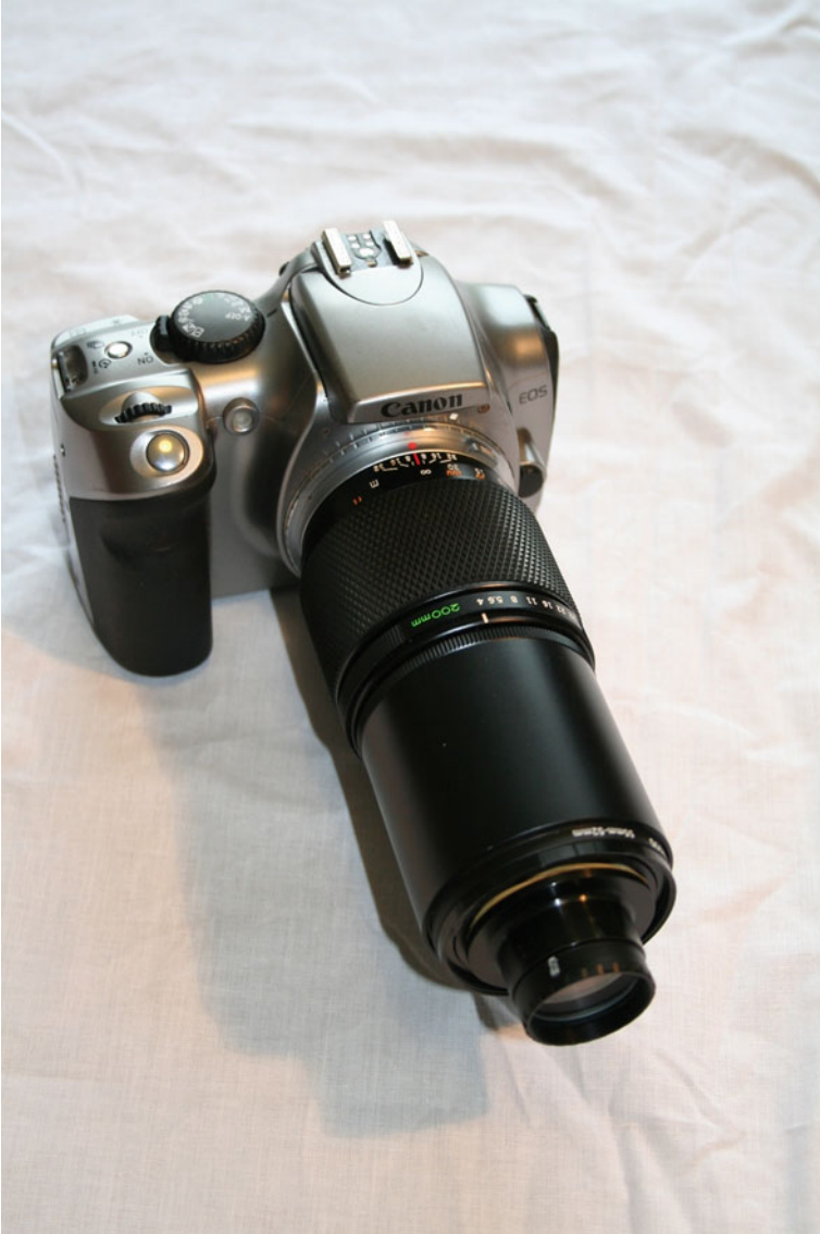
Figure 14.1. SA100 objective grating mounted on 200 mm telelens.
