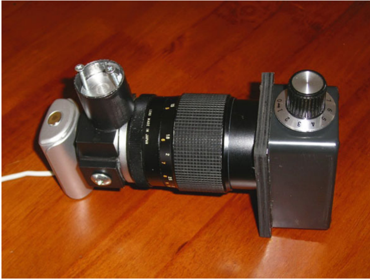
Figure 15.13. Compact WPO spectrograph.
