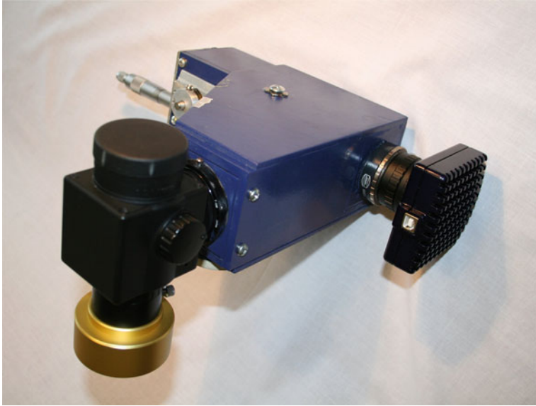
Figure 16.6. The beamsplitter and QHY5 guide camera in position on a Littrow spectroscope.
