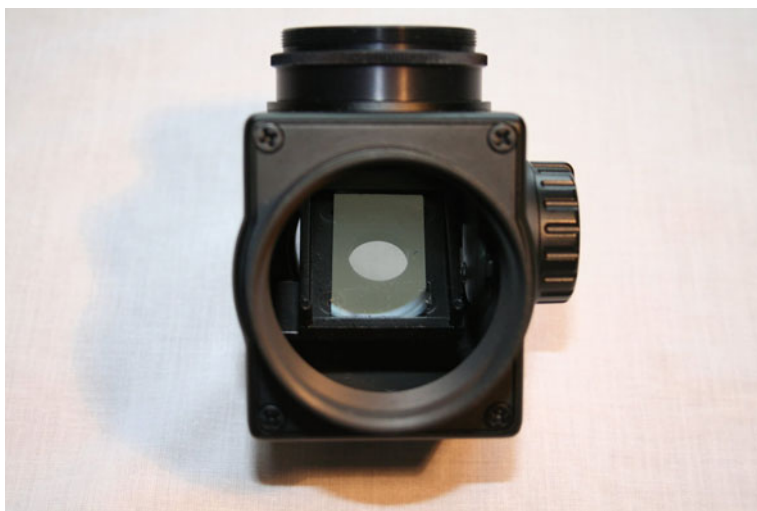
Figure 16.4. Beamsplitter in place.
