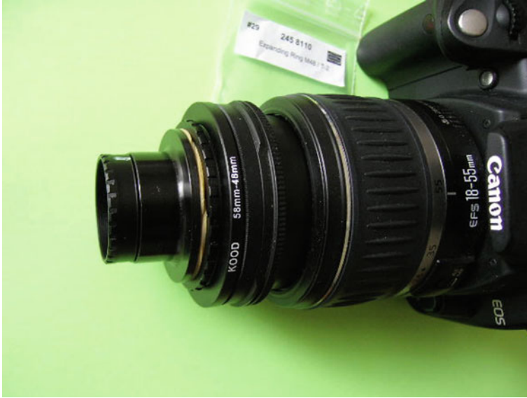
Figure 6.3. Filter grating mounted on camera lens.
