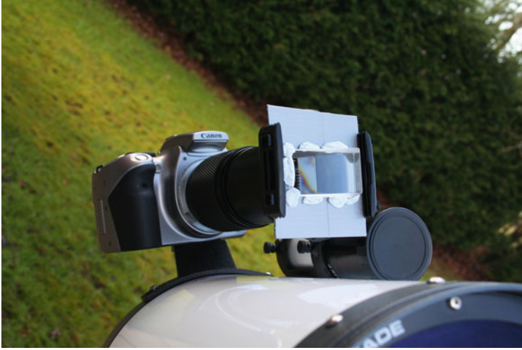
Figure 13.1. A 20° objective prism mounted in a Cokin filter adaptor.
