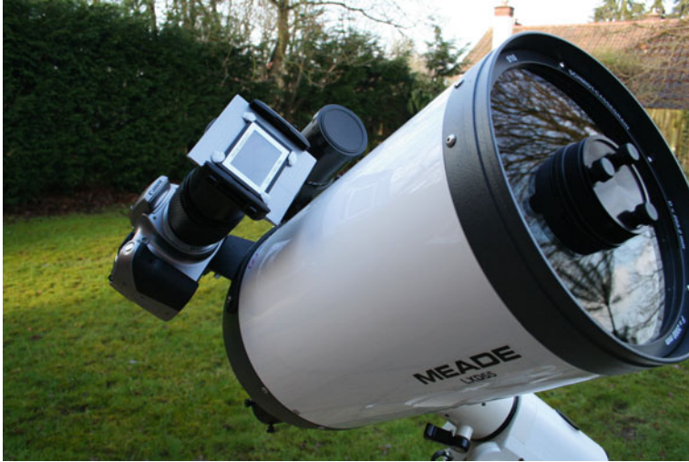
Figure 14.2. P-H objective grating mounted in a Cokin filter holder.
