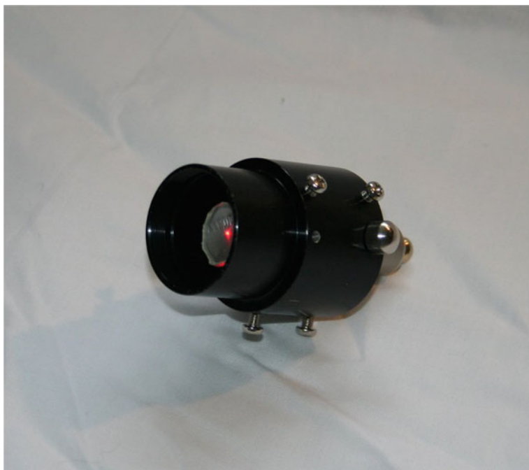
Figure 12.18. Homemade laser collimator.
