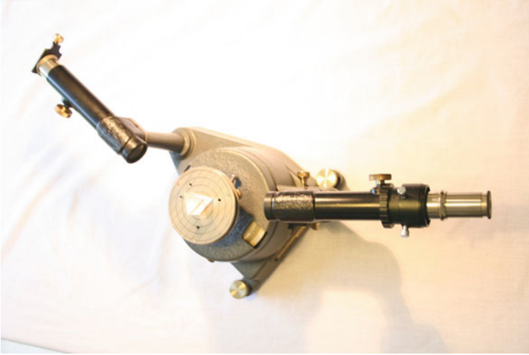
Figure 13.7. Standard school spectroscope layout showing the slit and collimator on the LHS, prism table center, and imaging telescope on the RHS.
