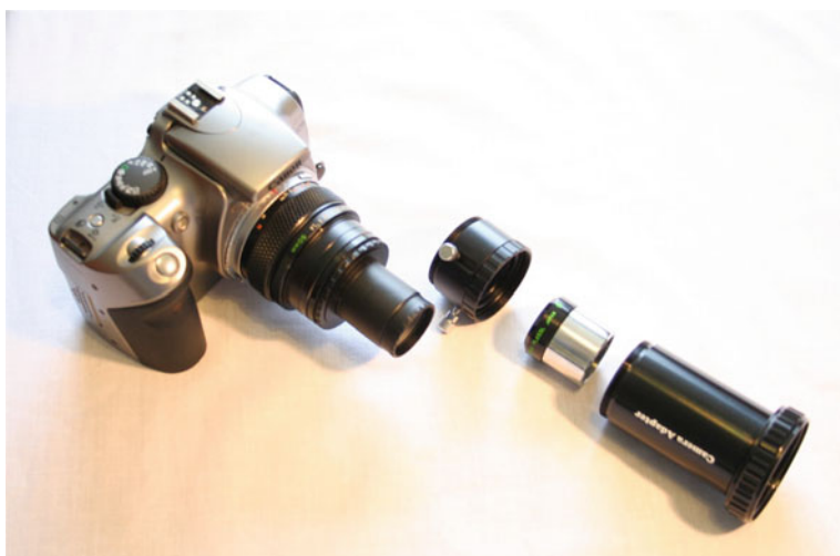
Figure 7.5. Eyepiece projection with filter grating, showing the components.
