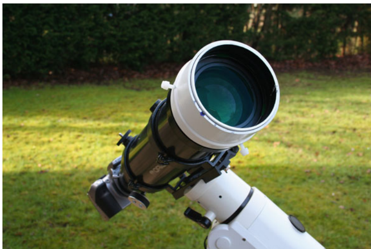
Figure 13.3. A 4^\circ objective prism on an ED80.
