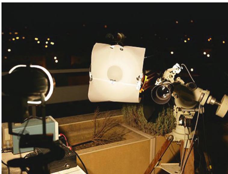
Figure 9.7. Taking a flat with a diffuser and halogen lamp. (C. Buil.)
