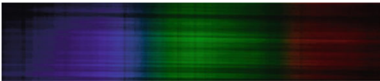
Figure 12.4. Transversalium lines showing on spectrum due to dirty entrance slit.
