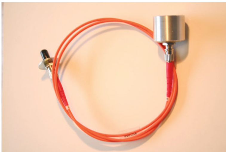
Figure 15.17. Standard fiber optic cable fitted to 1.25" nosepiece.
