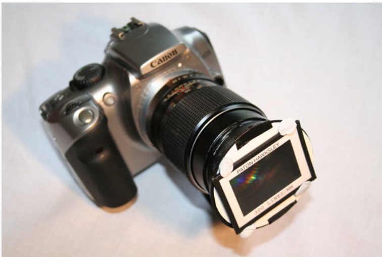
Figure 6.6. P-H grating mounted on a 135 mm telelens.
