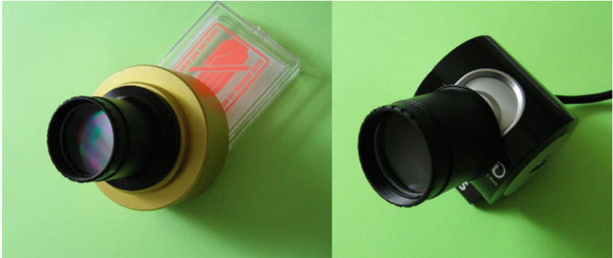
Figure 7.1. Filter gratings fitted to a QHY5 camera and a Philips SPC900 webcam.
