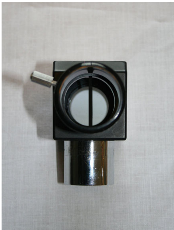
Figure 16.9. Split mirror guider.
