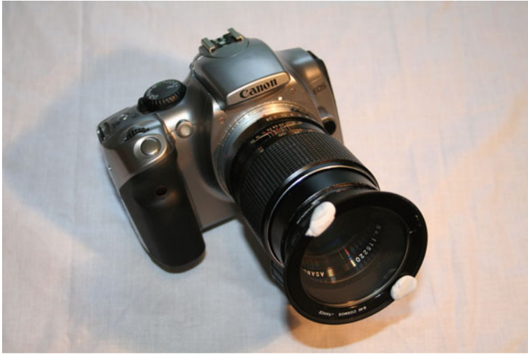
Figure 6.5. Cokin Cosmos grating filter mounted in lens hood of a 135 mm telelens.
