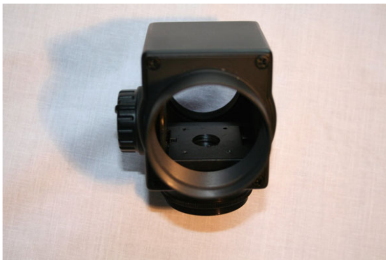
Figure 16.5. Rear view, showing the four small adjusting screws and the hole.
