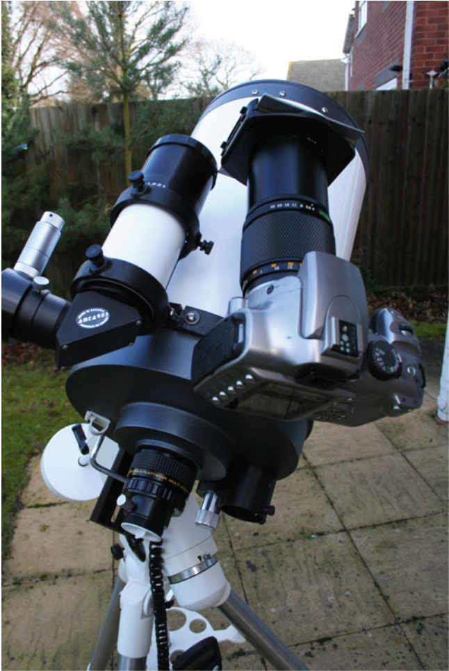
Figure 6.4. Objective prism mounted on a piggyback camera. Note the off-set angle.
