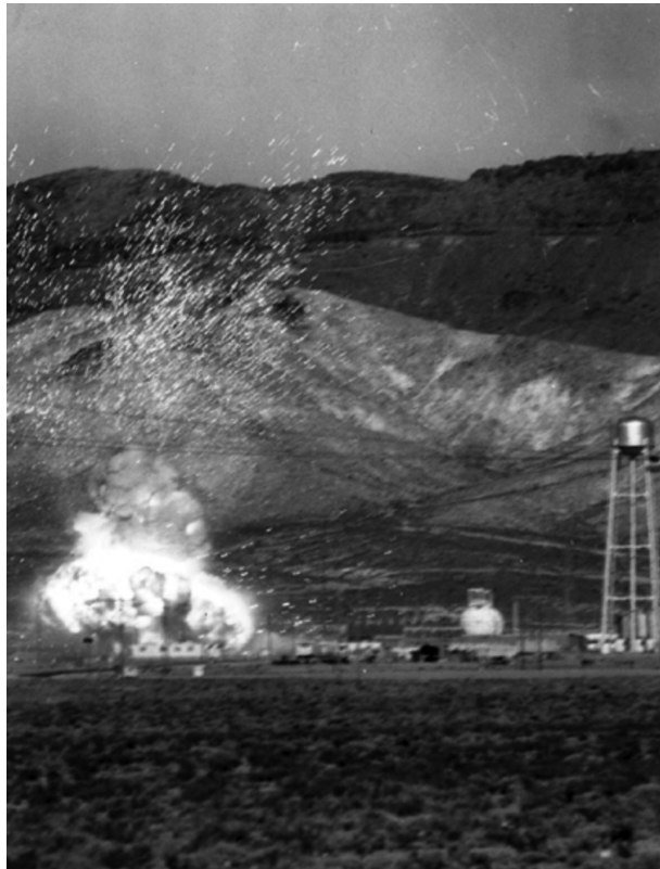
FIGURE 6.51 Destructive test of the Kiwi nuclear rocket engine reactor. (Courtesy of NASA.)
