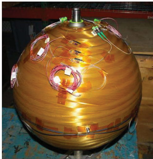
FIGURE 6.36 Space Shuttle OMS tank with stress sensors and circumference bulge gauges bonded to it. (Courtesy of NASA.)
