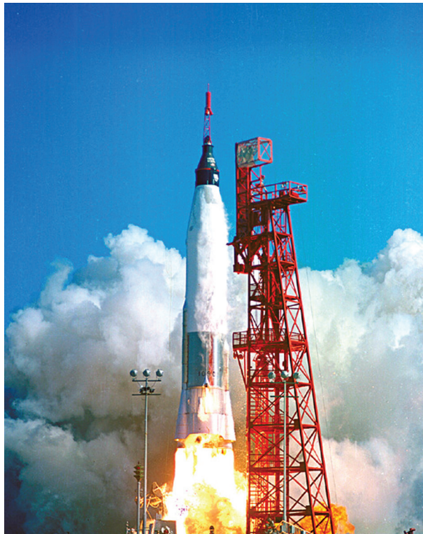
FIGURE 9.12 The Atlas rockets used monocoque propellant tanks to the dismay of the German rocket scientists. (Courtesy of NASA.)
