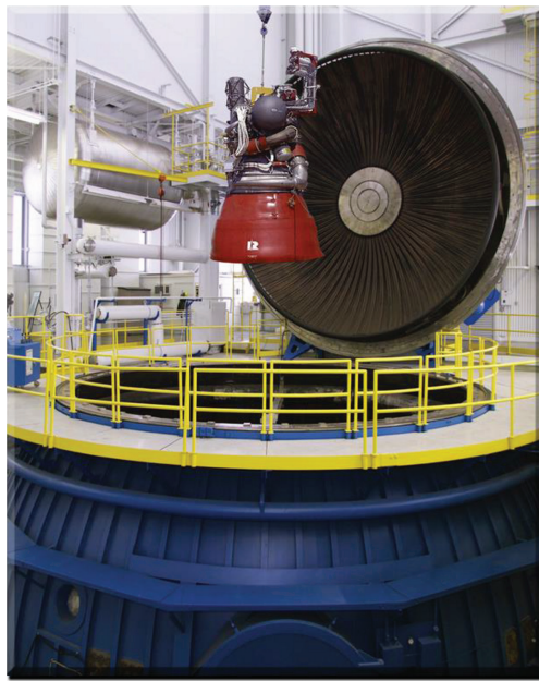
FIGURE 6.24 The J-2X engine being lowered into a vacuum chamber for testing. (Courtesy of NASA.)
