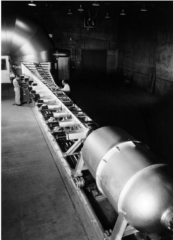
FIGURE 6.47 The Atmospheric Entry Simulator at NASA Ames (Mountain View, California). (Courtesy of NASA.)
