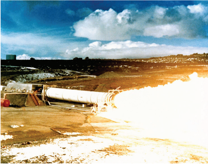
FIGURE 6.17 A solid rocket booster firing on the T-97 test stand. (Courtesy of NASA.)
