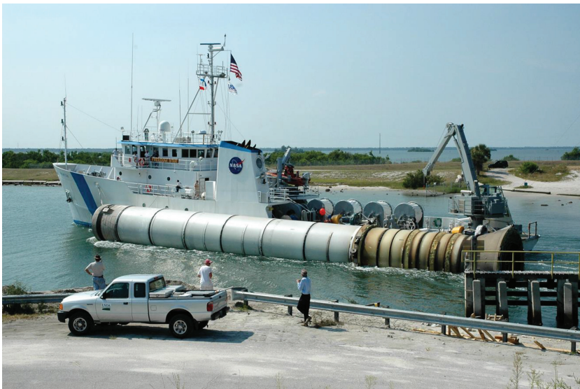
FIGURE 5.3 Space Shuttle SRB reusable casing retrieval from the ocean. (Courtesy of NASA.)
