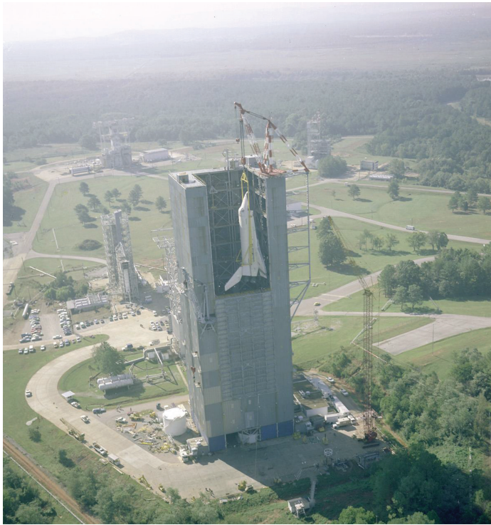
FIGURE 6.41 Space Shuttle Orbiter being loaded onto the MSC Dynamic Test Stand for Mated Vertical Ground Vibration testing. (Courtesy of NASA.)
