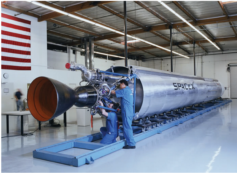
FIGURE 9.11 Falcon 1 uses monocoque propellant tanks.
