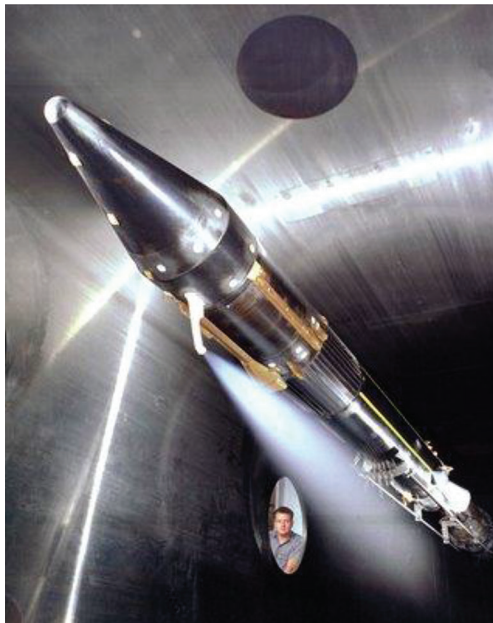
FIGURE 6.45 Supersonic wind tunnel testing of the Centaur rocket design. (Courtesy of NASA.)
