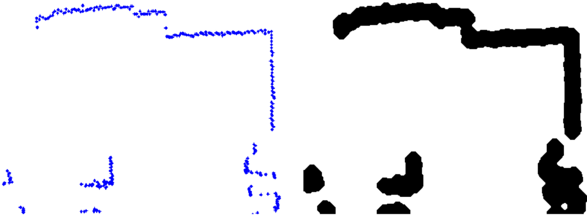
Figure 5. Data read by the robot (Local map) (left) Raw laser data (right) Thickened laser data
