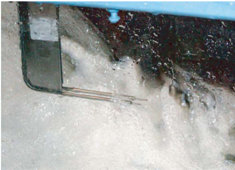
(b) Photograph of two single-tip conductivity probes side-by-side in a hydraulic jump ( Fr_1 = 7.9 , \rho_w * V_1 * d_1 / \mu_w = 9.4 E + 4 )—flow from right to left
