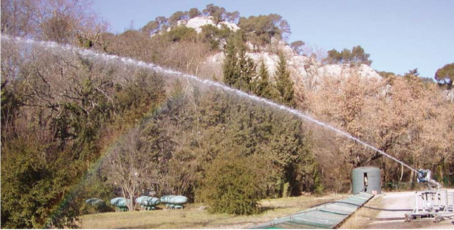
(C) Circular water jet (irrigation water canon)— d_1 = 0.0275 m, V_1 = 22.5 m/s, high-shutter speed (1/1,000 s)
