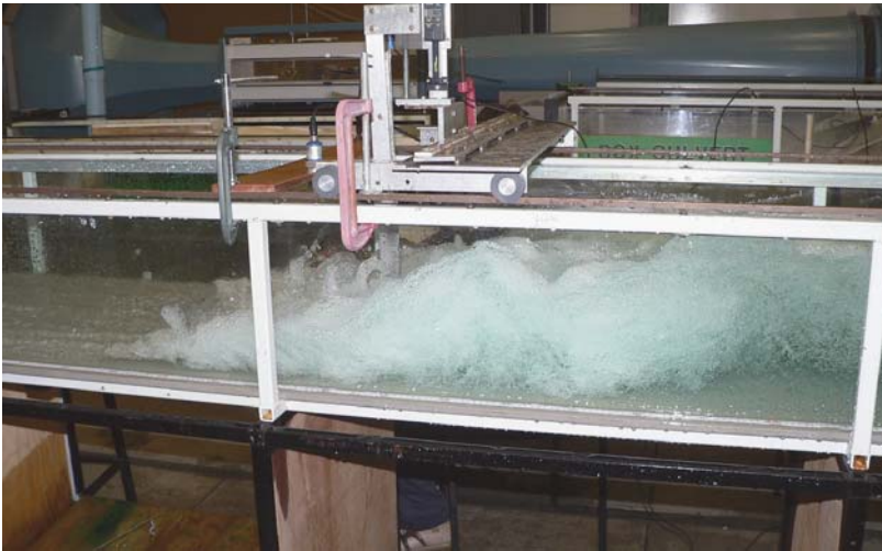
(B) Hydraulic jump in a rectangular channel ( V_1/\sqrt{g*d_1} = 7 , \rho_w * V_1 * d_1 / \mu_w = 8.1 E+4 ) —Flow from left to right
