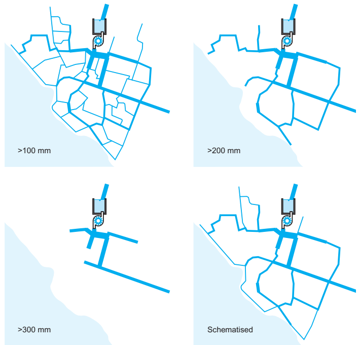
Figure 4.24. Example of network schematisation.
