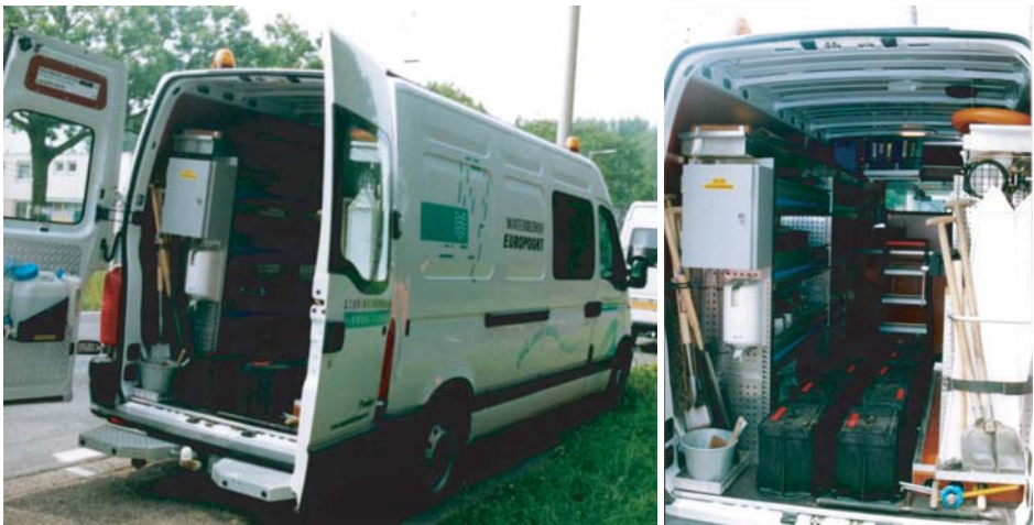
Figure 6.44. Mobile workshop for quick repair service.
