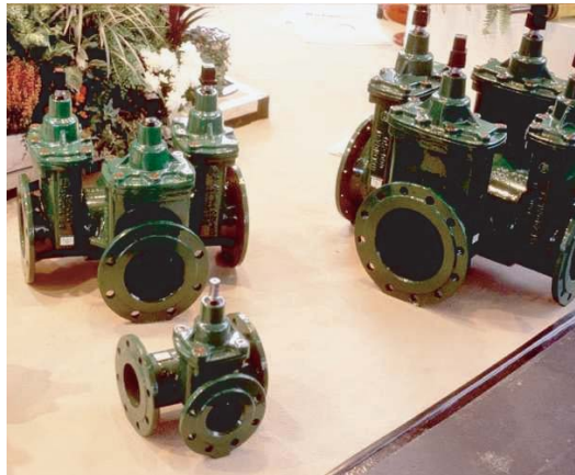
Figure 4.51. Blocks of gate valves.
