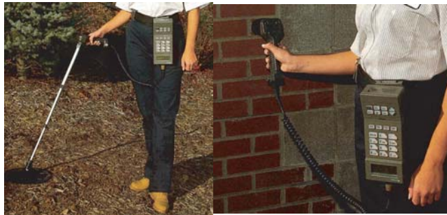
Figure 4.65. Automatic water meter reading (Manufacturer: Sensus).
