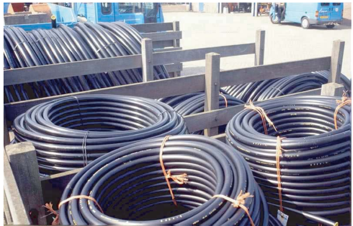
Figure 4.42. Stock of coiled PE pipes.
