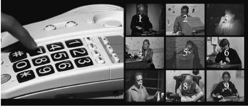
Figure 2 The Crossed Lines telephone interface: the telephone keys numbered 1–9 simply map on to the nine screens.
