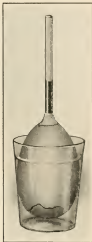
FIGURE 1. — SIMPLE OSMOMETER SHOWING OSMOSIS.
