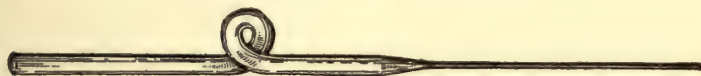
FIG. 9.—Coiled pipette for taking up small quantities of fluids. Bubbling in the coil gives warning of the filling and prevents suction into the mouth. The tube may be made straight and plugged with cotton. Either may be used for withdrawing serum from the Wright pipette. Suction may be applied by the mouth directly or with a rubber tube or by means of a small nipple.
