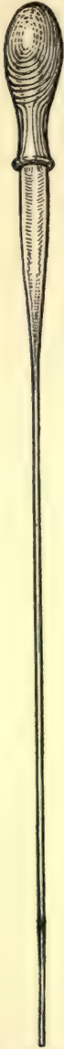
FIG. 11.—The nipple pipette for making mixtures of fluids and bacterial suspension. The pencil mark is seen a short distance above the tip.
