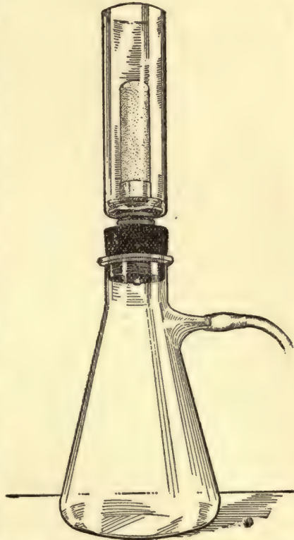
FIG. 1.—Apparatus for filtration through porcelain of small quantities of material. Between the rubber tube and the suction apparatus must be inserted a small trap to prevent entrance into the flask of water when suction is released. The trap is a salt neck bottle with an inlet and outlet tube through a rubber stopper.
