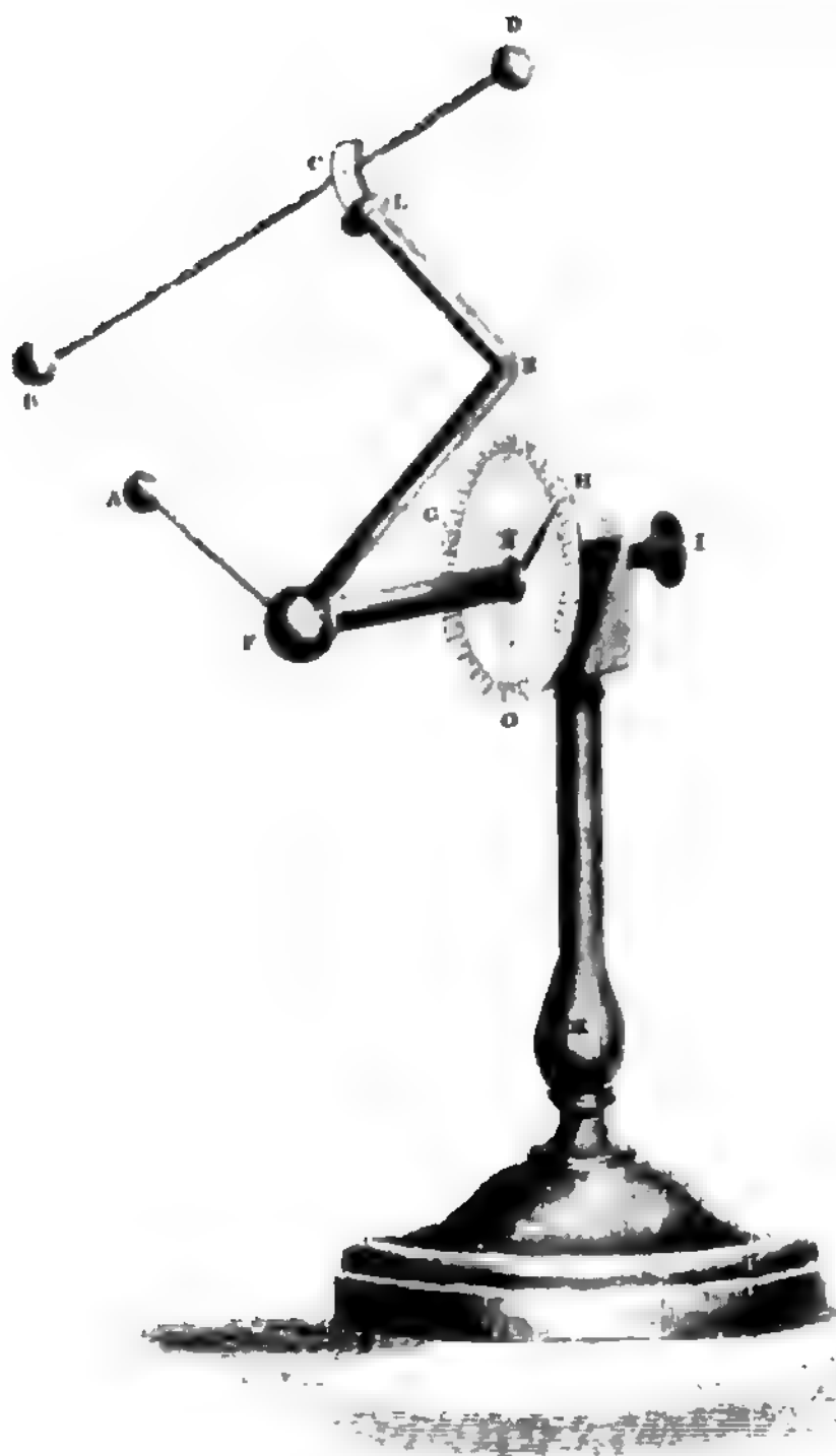
3.27 Robison's apparatus for measuring f(r) between small charged spheres. From Robison, System , IV (1822).
