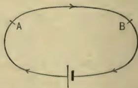
FIG. 403.—Diagram to illustrate Ohm's law.
