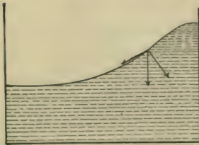
FIG. 82. — Forces acting at any point of the surface of a liquid when it is not horizontal.
