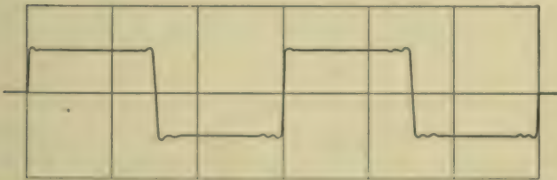
Composition of 100 harmonic vibrations whose periods are proportional to 1, \frac{1}{2} , \frac{1}{3} , etc., and whose amplitudes are proportional to 1, \frac{1}{2} , \frac{1}{3} , etc.
