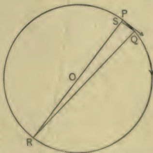
FIG. 23. — Uniform motion in a circle considered as a composition of uniform tangential motion and constant radial acceleration.
