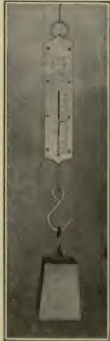
FIG. 29. — Spring Balance used for measuring weights.
