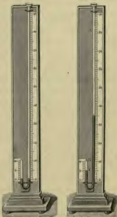
FIG. 97. — Apparatus for observing Boyle's Law; a small quantity of air is trapped in the closed end of the tube.
