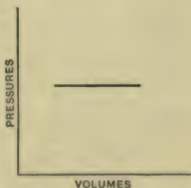
FIG. 129. — Isothermal of saturated vapor.
