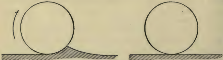
FIG. 59. — As a body rolls on a plane surface, both are deformed slightly.
