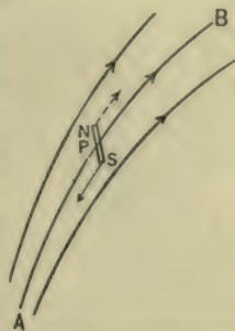
FIG. 315. — Lines of magnetic force, and the forces acting on a small magnet.
