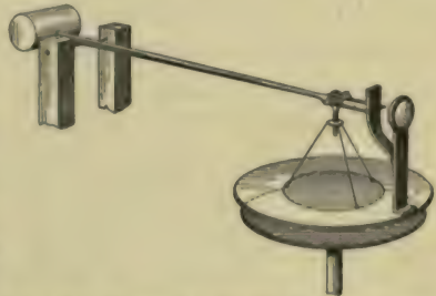
FIG. 856. — Thomson's original form of absolute "trap-door" electrometer.
