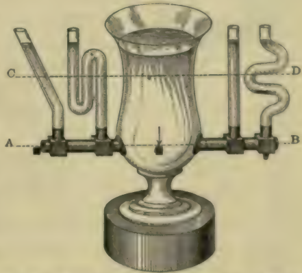
FIG. 86. — Same liquids in connecting tubes. AB and CD are horizontal planes.
