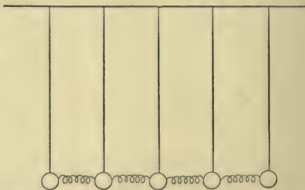
FIG. 147. — A ball and spring model for illustrating wave motion.
