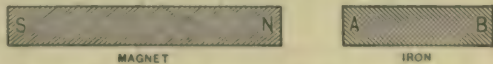
FIG. 306. — Magnetic Induction: the end A of the iron bar becomes a south pole.
