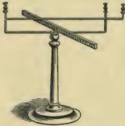
FIG. 361. — Apparatus of Oersted for studying the action of an electric current upon a magnet.
