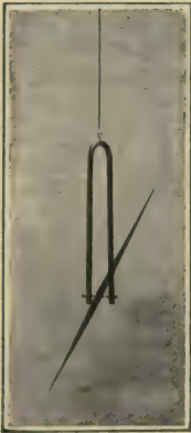
FIG. 324. — A magnetic needle suspended free to turn in any direction.
