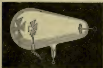
FIG. 883. — Shadow of maltese cross produced by cathode rays.
