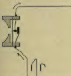
FIG. 397. — Diagram of Blake transmitter.
