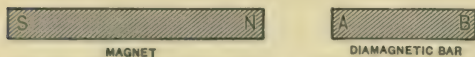
FIG. 322.—Action of a magnet on a diamagnetic body: A becomes a north pole.
