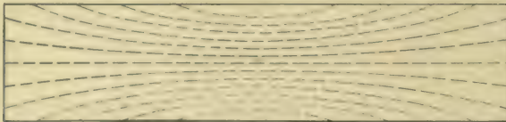
FIG. 311. — Diagram representing arrangement of molecular magnets in a bar magnet.
