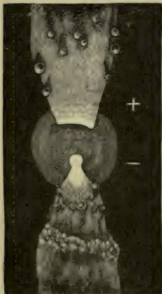
FIG. 358. — The electric arc between two carbon poles.
