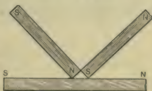
FIG. 309. — Process of magnetizing an iron bar by means of two magnets.
