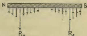
FIG. 312. — Forces acting on a bar magnet owing to a distant magnet.
