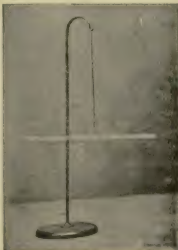
FIG. 330. — A glass rod suspended in a stirrup so as to be free to turn.
