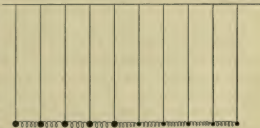
FIG. 148. — A model illustrating two media; in the one on the left the velocity of waves is less than in the one on the right.
